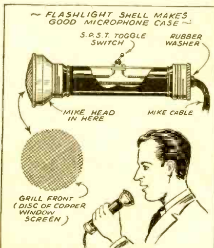
A simple microphone case made from a flashlight shell.
