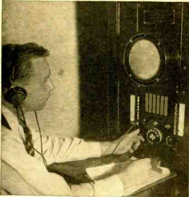
Photo above shows operator at airport checking direction of plane transmitting regular communication signal. The receiver employs an Azimuth-indicating device, operating in the 2 to 7 megacycle band. Right—Note size of man and the dipole antennas. Below—Diagram of receiver and arrangement of dipole antennas.
